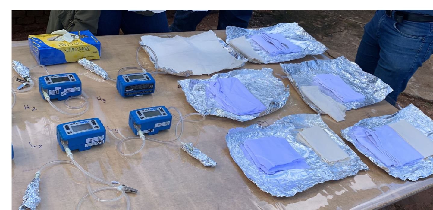
Weathering of dermal and inhalation dosimeters to be used as quality control
